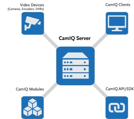
CamIQ Satellite reliably analyzes, records and transmits video data. Prevalent types of network cameras and appropriate video servers can be used as image sources.
